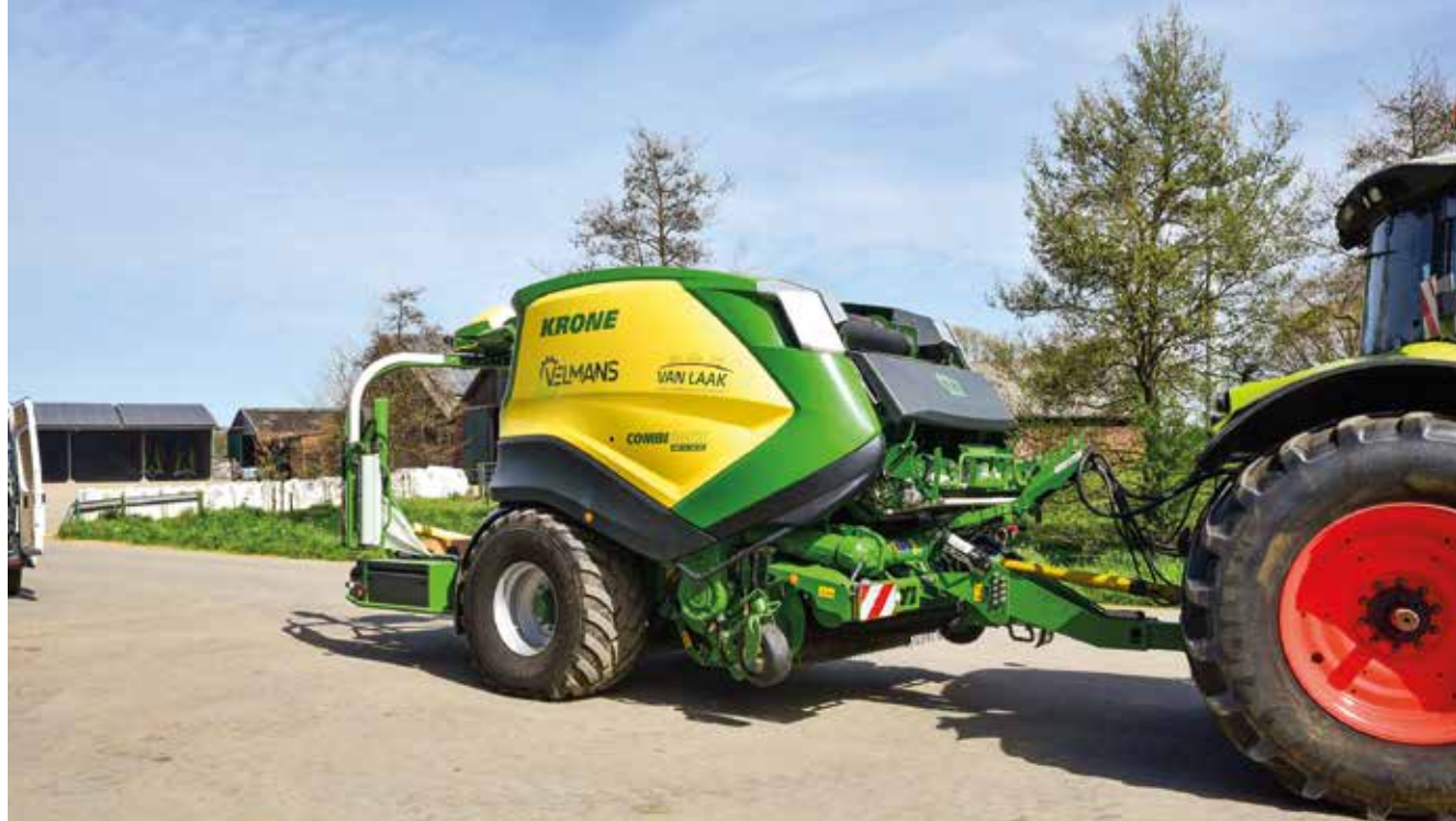
To get the most out of the KRONE Combi-Pack HDP 41-blade cutting unit, contractor Velmans uses a 300 hp tractor to pull it along.
