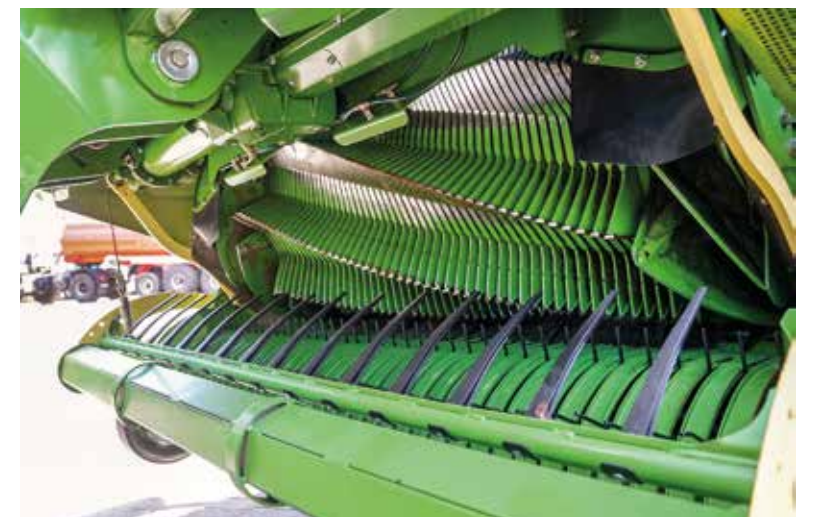
Centrepiece of the OptiGrass cutting unit: the integral rotor and SplitCut edge-cutting system ensure an even distribution in front of the blades and prevent excess lengths.
