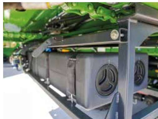
Optional feature: the 200 l silage additives tank.
