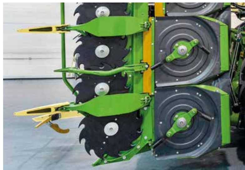
The flails on the mulching system are positioned so that they shred the stubble immediately after it has been cut.
