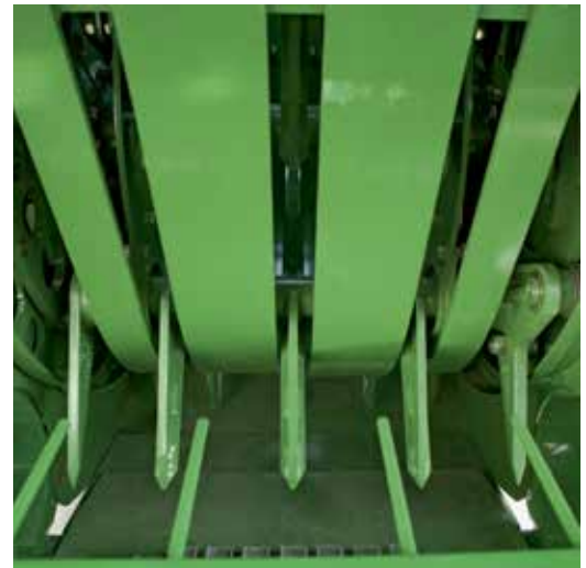
Fig. 3: Only when the feed chamber is filled to capacity does the retainer hook automatically swing to the rear. This clears the transition into the bale chamber and at the same time releases a clutch.
