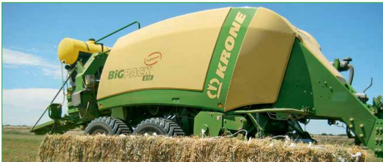
BiG Pack 870 from KRONE makes our unique MultiBale technology available in a smaller format. The machine produces regular big bales but can also tie up to eight small bales into one large 2'7" x 2'3" package, baling at a density as high as that achieved by KRONE BiG Pack 1290 HDP only and using our well-proven double knotter technology, which ties five threads of twine around the individual bales to form one large and firm package.
