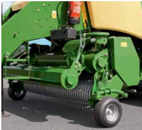
The new 'Active Pick-up' has a powered feed roller, which actively feeds the crop into the baler. The camless technology provides a number of obvious benefits: extremely quiet running and much higher throughputs whilst minimizing the number of moving parts.
